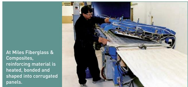
At Miles Fiberglass & Composites, reinforcing material is heated, bonded and shaped into corrugated panels.
